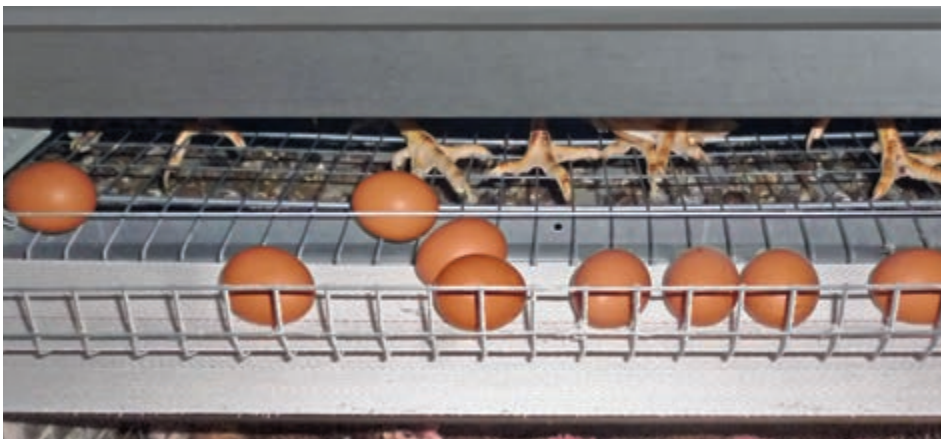
EggSaver in lowered position, carefully slowing down the eggs
