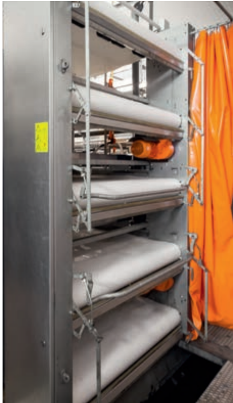
Manure belt end set with scrapers and central adjustment
