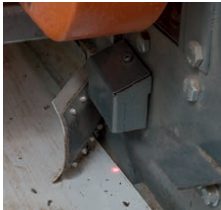
Light sensors monitor the belts
